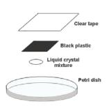
Use a wood applicator stick to place a small amount of the liquid crystal mixture to the inside of a Petri dish. Place a piece of black plastic, approximately 2.5 cm square, on top of it and seal it in place with a 5 cm square of clear plastic shipping tape.
