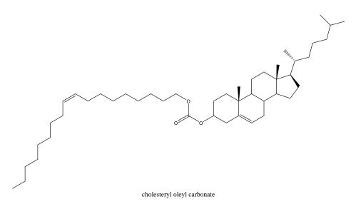
These cholesteric-nematic liquid crystals reversibly change color as the temperature changes. One of the principal advantages of liquid crystals is their ability to map out thermal regions of different temperature. Liquid crystal films exposed to the atmosphere will decompose slowly; their lifetime can be extended by encapsulation.
