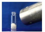
Melt the solid in a sample vial using a heat gun.
